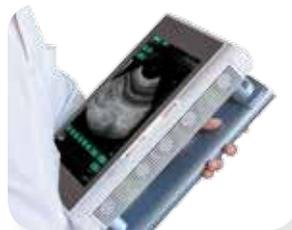
Built-in transducer controls
